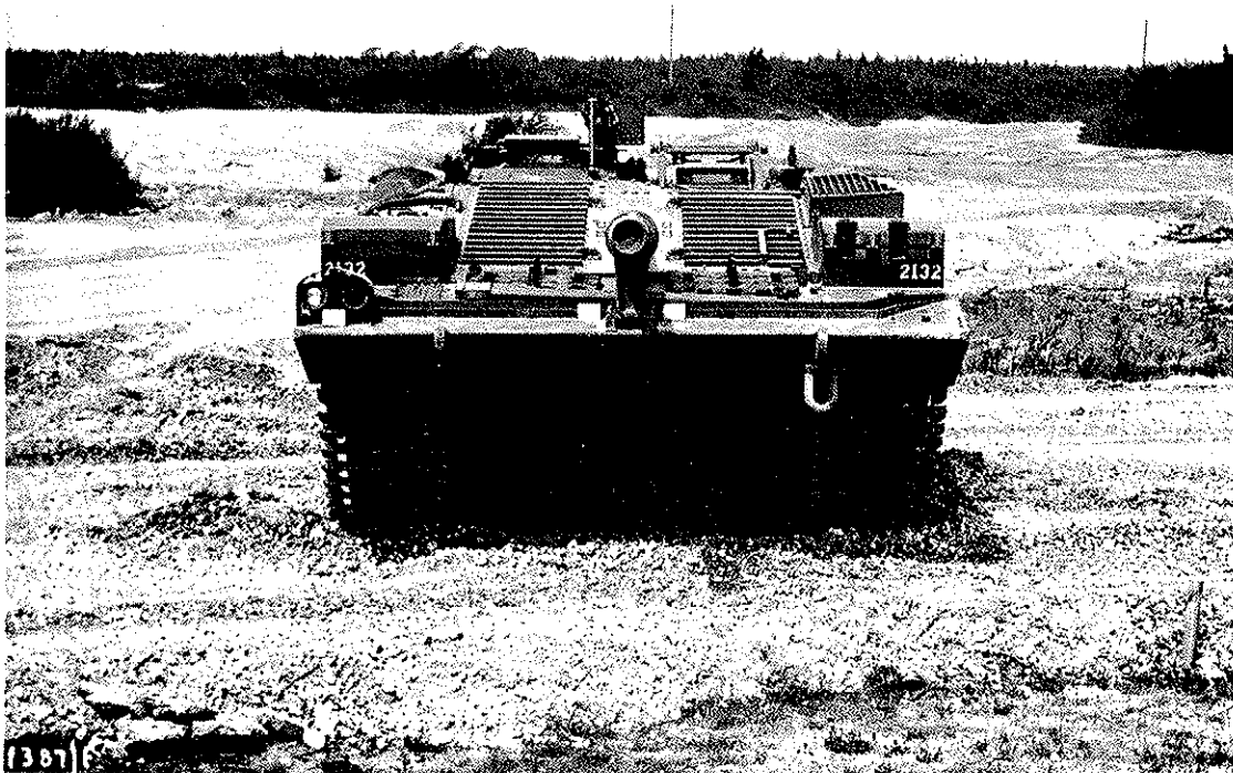
Plate 1 'S' TANK - FRONT VIEW
