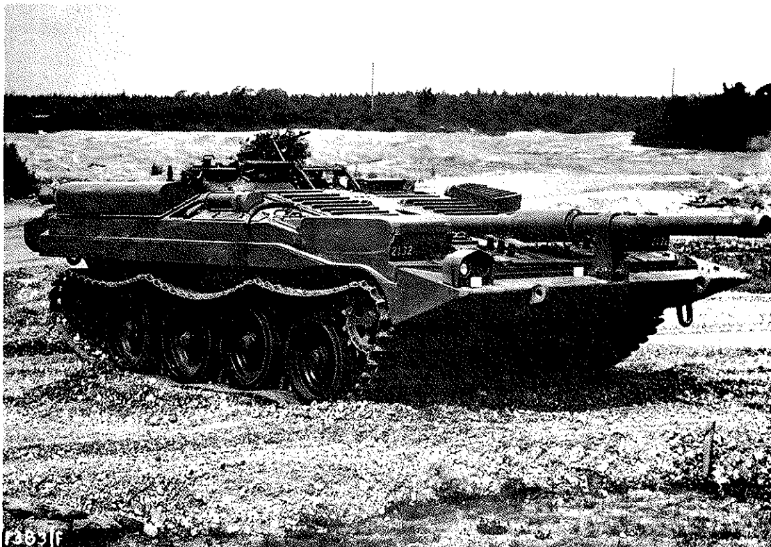
Plate 8 'S' TANK - RIGHT HAND FRONT \frac{3}{4} VIEW, SUSPENSION IN THE LOWERED POSITION
