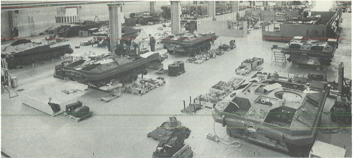
Beginning of the assembly of S-tanks at Bofors.
