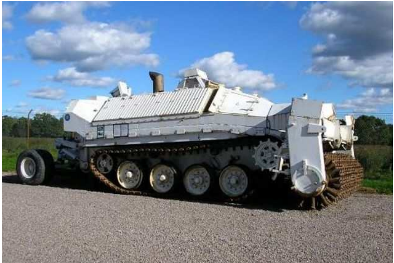
MV 103 C Deminer – Army Camp, Skillingaryd. (Sweden) Stridsvagn Strv 103C (202232) modified into land mine clearing vehicle
